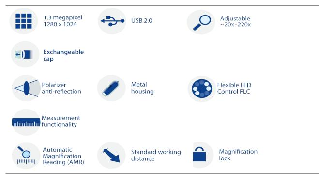
The AMR function automatically detects and displays the magnification of the Dino-Lite. The magnification is displayed within the Dino-Lite software and stored with the captured picture and simplifies the measuring process. Because of the built-in polarization filter this model is ideal when working with shiny or reflective objects such as metal, plastic, glass, jewelry, electronics, etc.
